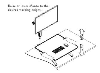
Adjust the height of Monto to a comfortable working height. There are a <u>total of 9 positions</u>.
